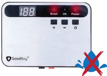
Power on, wire broken or not installed
